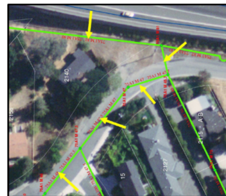
Figure 12: Parcel illustrating 5 mainline sewer segments that could have lateral connections to single structure
